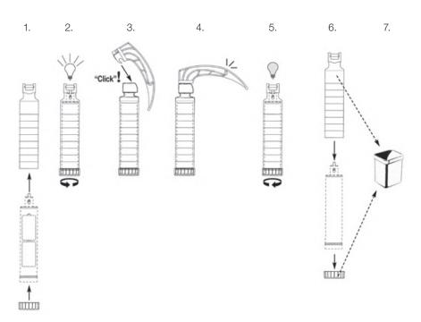
The XP disposable handle shell was especially designed for use with HEINE laryngoscope inserts. The HEINE laryngoscope insert is placed inside the disposable handle shell and the light is activated by turning the bottom insert. Following intubation, the user simply unscrews the bottom insert and the laryngoscope insert can be removed with no risk of contamination. The handle shell, the bottom insert and the XP blade are all disposed of.
